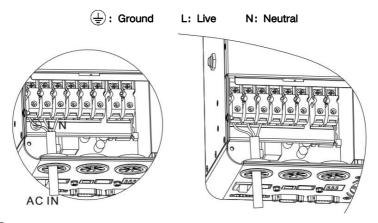
(3) Properly connect the AC output wire according to the wire sequence and terminal position shown in the figure below. Please connect the ground wire first, and then the live wire and the neutral wire. The ground wire is connected to the grounding screw hole on the cabinet through the O-type terminal.
