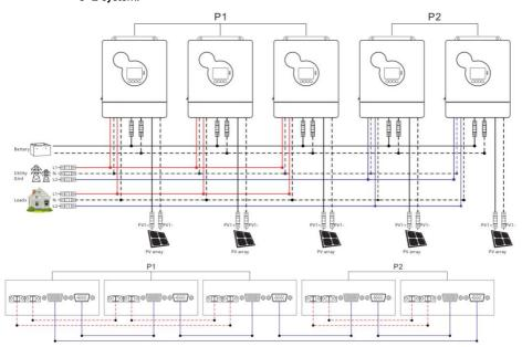
e) Six all-in-one solar charger inverters of the system connected in two phase:5+1 system:
