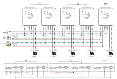
d) Six all-in-one solar charger inverters of the system connected in three phase:
