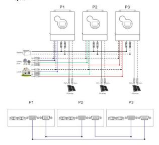
b) Four all-in-one solar charger inverters of the system connected in three phase:2+1+1 system:
