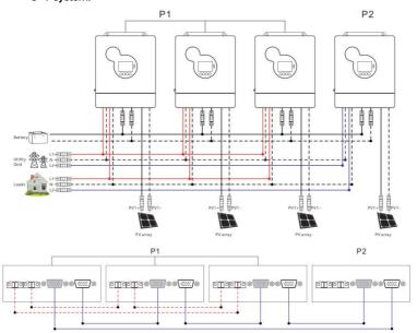
d) Five all-in-one solar charger inverters of the system connected in two phase:4+1 system:
