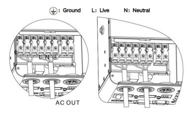
**Note:** The grounding wire shall be as thick as possible (cross-sectional area is not less than 4mm<sup>2</sup>). The grounding point shall be as close as possible to the all-in-one solar storage inverter. The shorter the grounding wire, the better.
