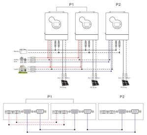
c) Four all-in-one solar charger inverters of the system connected in two phase:2+2 system:
