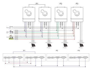
Five all-in-one solar charger inverters of the system connected in three phase:
