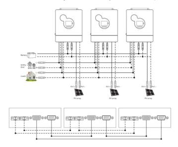
c) Four all-in-one solar charger inverters of the system connected in parallel:
